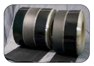
The 6" RMS strip may be installed either horizontally or vertically. The 6" RMS has a 3" wide In-seam tape preapplied to one edge. The EPDM field sheet is then seamed to the RMS. When using the RMS, Tape Primer must be used to prime the EPDM membrane.
