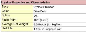
Typical properties and characteristics are based on samples tested and are not guaranteed for all samples of this product. This data and information is intended as a guide and does not reflect the specification range for any particular property of this product.
