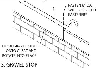
HOOK DRIP EDGE OF EACH GRAVEL STOP SECTION ONTO CONTINUOUS CLEAT, ROTATE INTO PLACE. FASTEN THRU PRE-SLOTTED HOLES 6" WITH PROVIDED FASTENERS.
