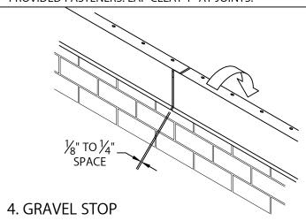
CONTINUE INSTALLING LENGTHS OF GRAVEL STOP. LEAVE A  $\frac{1}{8}$ " TO  $\frac{1}{4}$ " SPACE BETWEEN PIECES.
