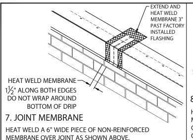
**HOT AIR WELD** ALONG LENGTH OF DRIP EDGE APPLY CUT EDGE SEALANT ALONG EDGE IN AREAS OF PONDING **WATER ONLY** 8. FLASHING
