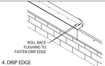
ROLL BACK FLASHING TO EXPOSE FASTENING SLOTS AND FASTEN THRU PRE-SLOTTED HOLES 6" WITH PROVIDED FASTENERS.
