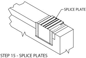
PLACE SPLICE PLATE ONTO ANCHOR CLIPS AT SPLICE JOINTS.
