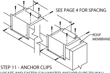
LOCATE AND FASTEN GALVANIZED ANCHOR CLIPS TO WALL AT CENTERS WITH PROVIDED FASTENERS FOR SUBSTRATE SEE
