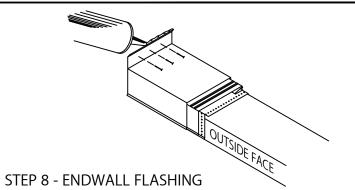
FASTEN TO WALL USING APPROPRIATE FASTENERS AS SHOWN. APPLY NON-CURING SEALANT (BY OTHERS) TO CAULK CUP ATOP 3" FLANGE.
