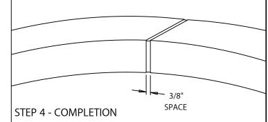
NOTE: REMOVE PROTECTIVE FILM IMMEDIATELY. USING ARCHED SECTIONS TO COVER WALL CONDITIONS, CUT TO LENGTH AS NEEDED USING A FINE TOOTH HACKSAW, SNIPS, OR CUT-OFF WHEEL LEAVING A CLEAN EDGE.
