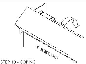
HOOK OUTSIDE FACE OF COPING OVER THE ANCHOR CLIP/ENDWALL FLASHING AND ROTATE INTO PLACE. ENGAGE REAR LEG ONTO ANCHOR CLIP BY PRESSING DOWNWARD UNTIL SNAP LOCK OCCURS.
