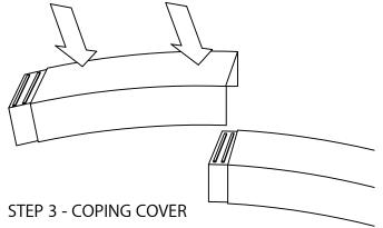
PLACE COPING INTO POSITION ALLOWING 3/8" SPACE AT SPLICE JOINT. FASTEN THROUGH TOP OF COPING AS SHOWN IN STEP #1
