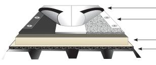
Fleece back (TPO, PVC or PVC KEE HP) Membrane Existing aged Single-ply (EPDM, TPO Hypalon)<sup>1,2</sup> or existing modified asphalt system<sup>1,3</sup>
