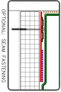
OPTIONAL: SEAM FASTENING PLATE/FASTENER MAY ALSO BE INSTALLED INTO THE STRUCTURAL DECK.
