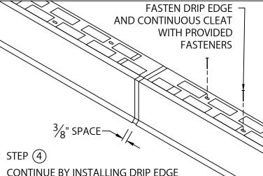
CONTINUE BY INSTALLING DRIP EDGE SECTIONS ALLOWING A 3/8" SPACE BETWEEN SECTIONS AS SHOWN. FIELD CUT AS NECESSARY. REMOVE PROTECTIVE FILM IMMEDIATELY AFTER INSTALLATION. INSTALLERS SHALL WEAR PROTECTIVE EYEWEAR TO PREVENT INJURY.
