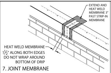
HEAT WELD A 6" WIDE PIECE OF NON-REINFORCED
