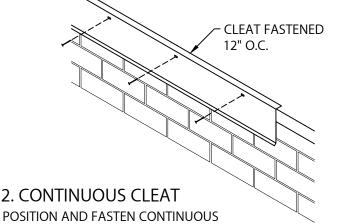
POSITION AND FASTEN CONTINUOUS CLEAT 12" O.C. THRU PRE-SLOTTED HOLES AS SHOWN WITH PROVIDED FASTENERS. LAP CLEAT 1" AT JOINTS.
