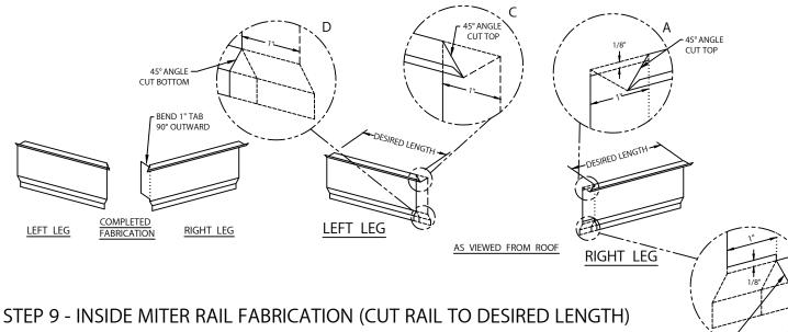
RIGHT LEG - DETAIL A: FIRST REMOVE SECTION 1/8" DOWN FACE AND 1" HORIZONTALLY AS SHOWN TO CREATE TAB. TRIM TOP FLANGE BACK AT A 45° ANGLE. DETAIL B: CUT OFF BOTTOM FACE 1/8" AS SHOWN AND CONTINUE CUT AT A 45° THROUGH AREA SHOWN ON
