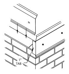
STEP 3 - RAIL MITER PREPARATION SEE PAGE 4 FOR MITER PREPARATION. FASTEN MITER BASE RAIL TO NAILER(S) THROUGH BASE RAIL SLOTS WITH PROVIDED FASTENERS.
