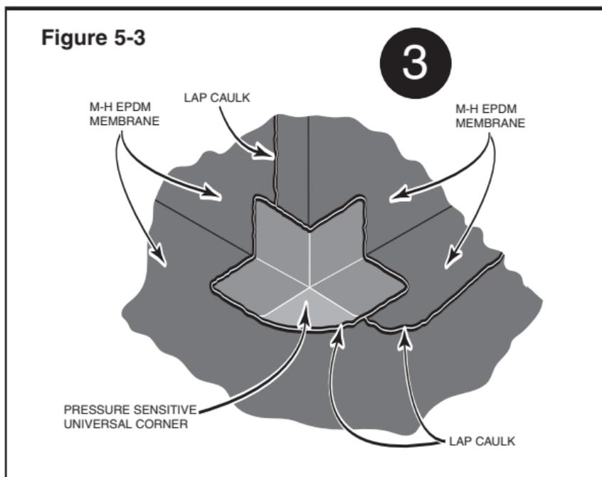
Repeat the same procedure with each outside corner. After about two hours or at the end of the day, apply a bead of Lap Sealant to all flashing edges. Again, it is not necessary to trowel or feather the Lap Sealant. Each corner should be completed in this manner.
