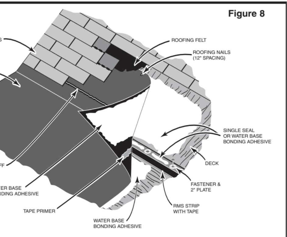
4. Chalk a line on the EPDM membrane for aligning the starter strip. Place a 3/8-inch bead of Water Cut-Off or Urethane Sealant approximately 2 inches to 3 inches above the chalk line and below the area where the nails will be driven to reinstall the starter strip. This will act as a seal for any water or ice backup. Reinstall the starter strip and shingles, running the nails through the Water Cut-Off.
