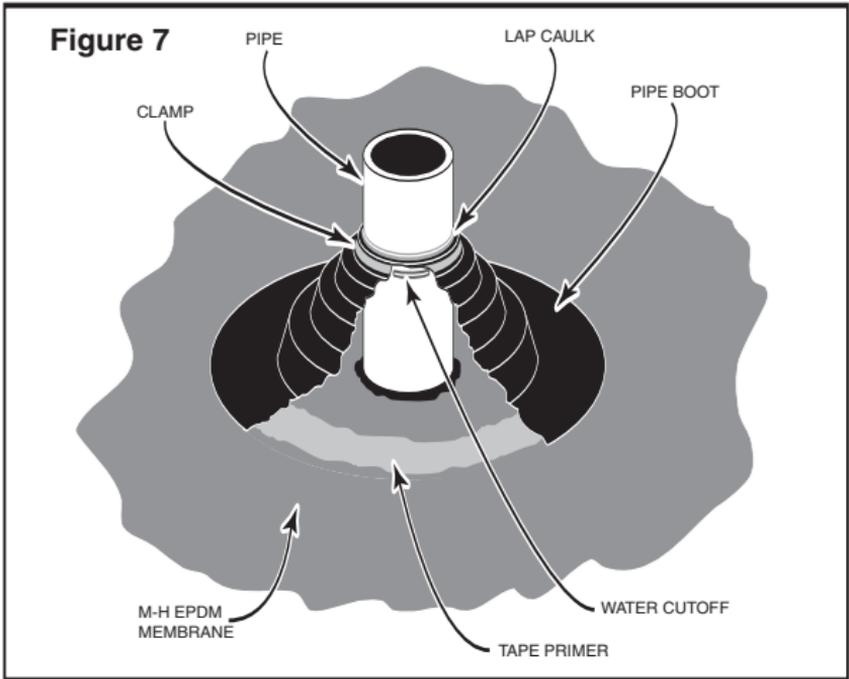
2. Using Mule-Hide Tape Primer, thoroughly clean the EPDM membrane around the pipe. Work the Tape Primer into the sheet with the Scotch-Brite® pad.
