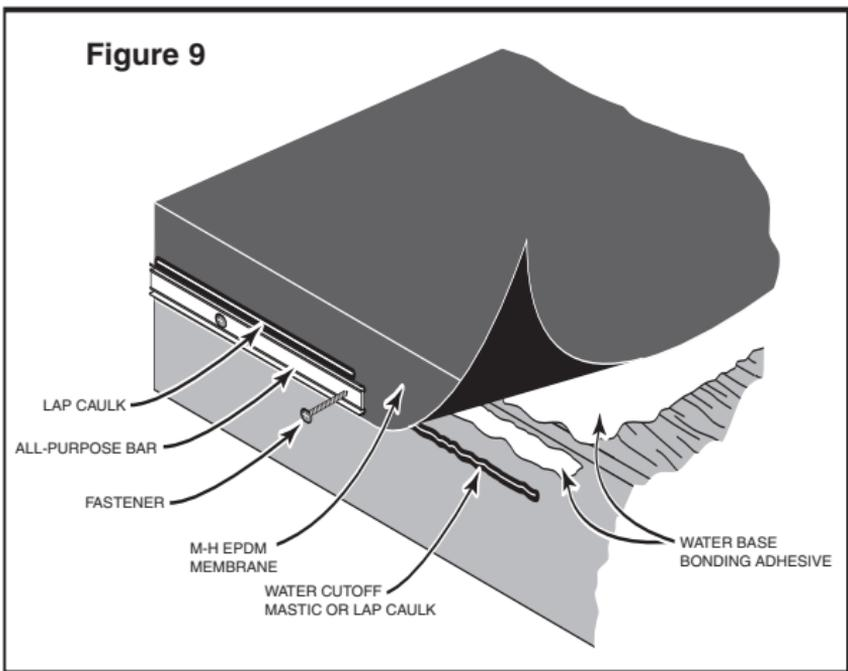
3. Roll the membrane back over the roof edge and install the All Purpose Bar using Mule-Hide Fasteners every 6 inches. Make sure that the two round or radius points on the All Purpose Bar are facing the fascia board. This will allow a lip for the lap caulk to be applied in step #4.
