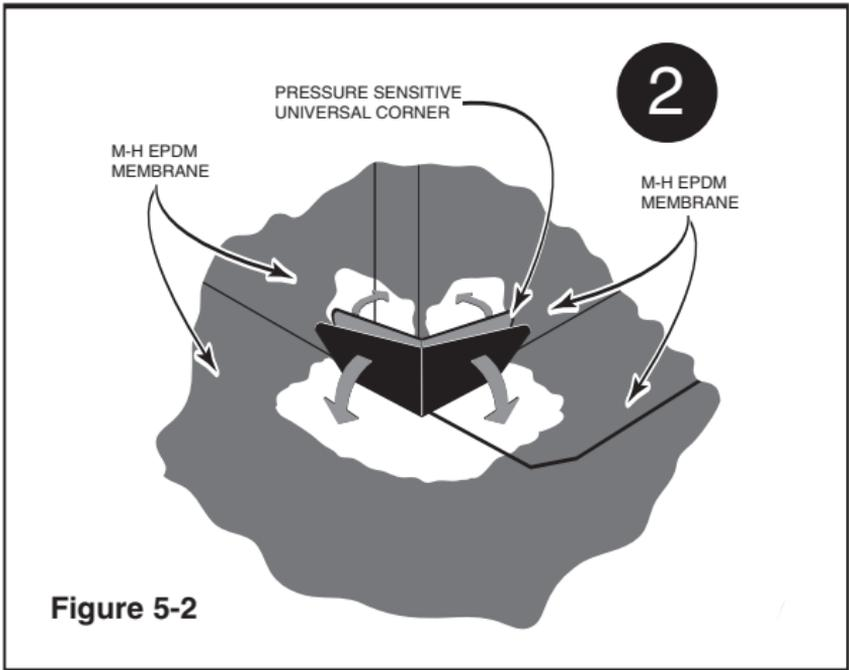
3. Remove the remaining release paper and form the flange out onto the horizontal surface by starting in the middle. Gently stretch the material so that the flashing can turn down onto the roof sheet without wrinkling and press into place. There should be no bridging in the corners or wrinkles. In colder weather, it may be necessary to warm the Pre-Cut Corner with a hot air gun to soften the material to allow for forming.
