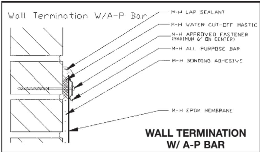
5. Fasten the All Purpose Bar to the wall with the Mule-Hide Fasteners spaced 6 inches on center. Trim off any excess membrane above the bar and apply a bead of Lap Sealant or Urethane Caulk along the top edge of the bar completing the detail. This detail should only be used on shiplapped wood siding, brick, or masonry surfaces. The EPDM sheet should be installed behind any vinyl siding or vertical wood siding. All old roofing materials must be removed before adhering the membrane to the wall.
