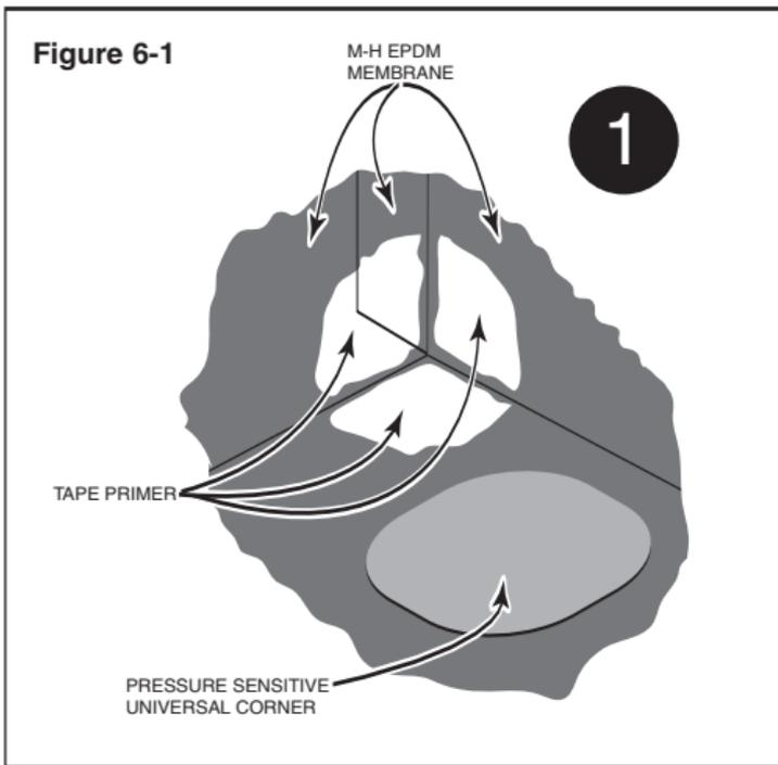
2. Position this piece in the corner so that the midpoint of the fold is tight to the corner with 4-1/2 inches extending up and 4-1/2 inches out onto the roof surface. Press into place. Remove the remaining release liner working the bottom half of the fold up the side of the wall. This will form a fold that is commonly referred to as a pig's ear. Press the fold together.
