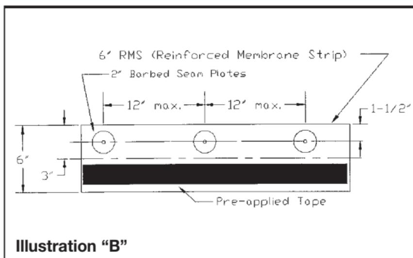
3. After the RMS Strips have been attached to the roof deck, position the field sheet to allow enough membrane to flash the vertical surface to the point of termination. Once the EPDM sheet is adhered to the roof surface, the EPDM sheet is rolled back to expose the RMS Strip. The EPDM sheet is cleaned with Mule-Hide Tape Primer, allowed to dry, and folded back over the RMS Strip.
