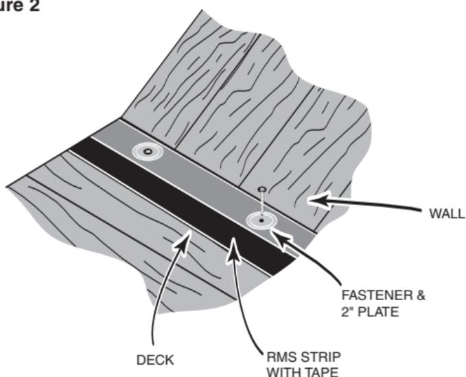
curbs, or shingle tie-ins. The RMS Strip is a reinforced EPDM strip that has a 3-inch wide butyl tape laminated to one side. The pre-applied tape helps speed up and simplify the installation process.
