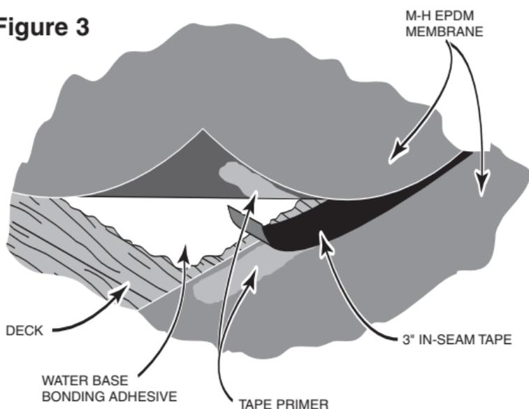
2. After folding back the top sheet, prepare each surface of the seam by scrubbing, using a circular motion, with Mule-Hide's Tape Primer and either clean cotton rags or Scotch-Brite, pads. The Scotch-Brite, pads are preferred for the application of the Tape Primer. Remember to replace the pads or rags with new ones once they become soiled. **Remember:** Both the underside of the top sheet and the topside of the bottom sheet must be scrubbed with the Tape Primer.
