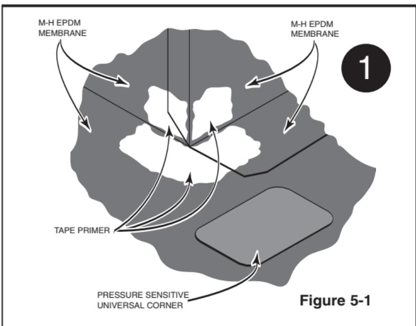
2. When the Tape Primer has dried, take the Pre-Cut Corner, fold in half, with the fold facing down and the bare tape facing the curb and apply the corner to the vertical surface of the curb so that it wraps each side of the corner about 3 inches. Press tightly in place.
