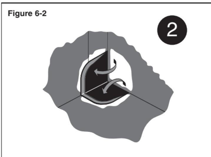
3. Apply Tape Primer to the fold and to the surface to which the fold will be adhered. When dry, cut a piece of 3-inch wide In-Seam Tape the length of the fold. Fit the tape between the pig's ear and the vertical wall. Remove the release liner and press the fold tight to the wall. Roll with a 2-inch steel roller.
