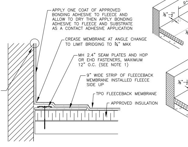
MINIMUM OF 2 BEADS MUST BE APPLIED TO TOP OF 9" FLEECEBACK STRIP TO ENSURE PROPER ADHESION OF FIELD MEMBRANE
