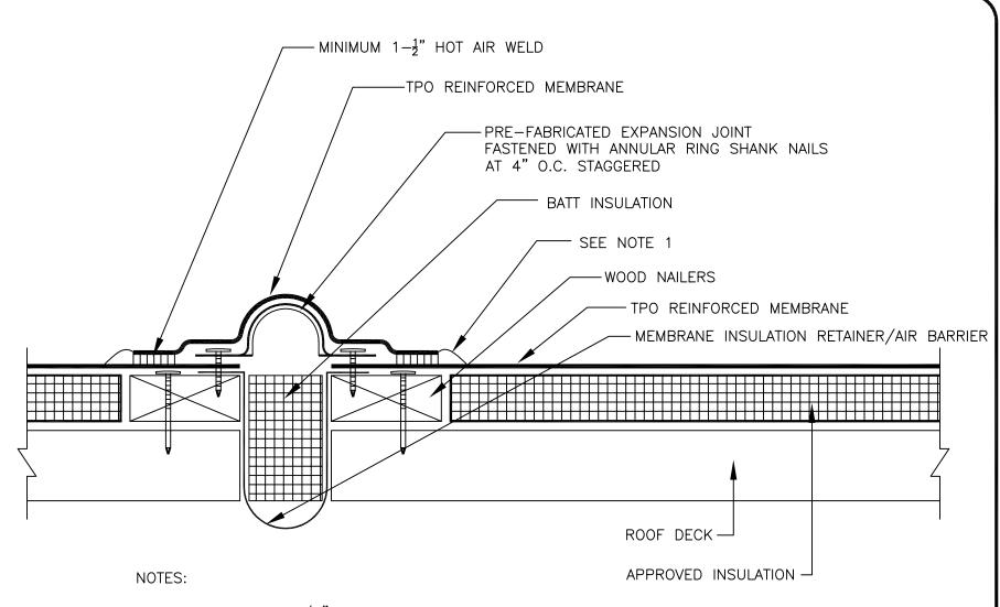
1. APPROXIMATELY 1/8" DIAMETER BEAD OF CUT-EDGE SEALANT IS REQUIRED ON CUT EDGES OF TPO REINFORCED MEMBRANE.
