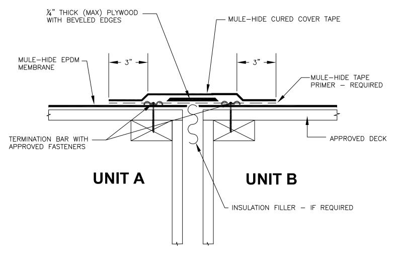
NOTE: DISTANCE FROM EDGE OF ROOF TO TERMINATION BAR SHALL NOT EXCEED 2 INCHES.
