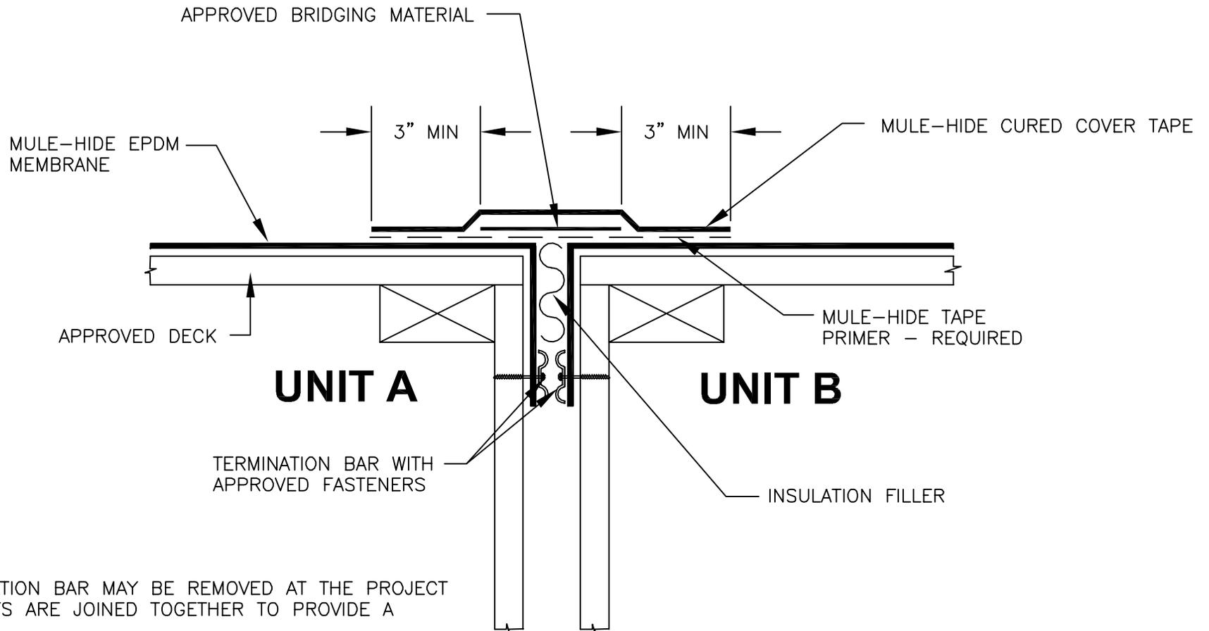
NOTE: TERMINATION BAR MAY BE REMOVED AT THE PROJECT SITE WHEN UNITS ARE JOINED TOGETHER TO PROVIDE A TIGHTER FIT.
