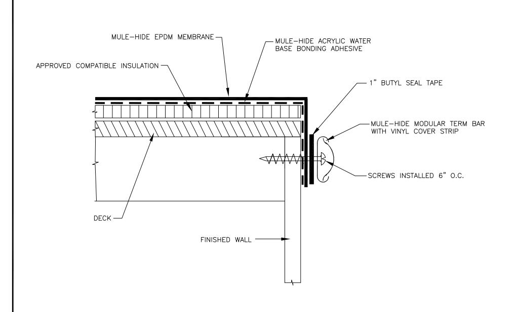
MULE-HIDE PRODUCTS CO., INC. 2010 EDGE TERMINATION BAR WITH COVER SYSTEMS: MODULAR SYSTEMS EPDM
