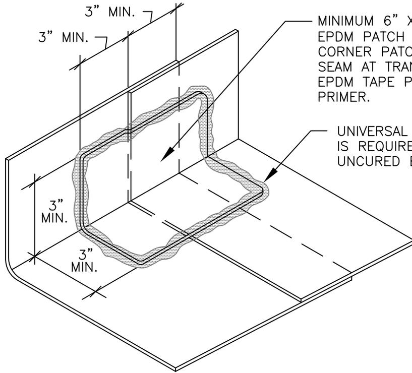
MINIMUM 6" X 6" WHITE UNCURED EPDM PATCH OR WHITE PRECUT CORNER PATCH CENTERED OVER SEAM AT TRANSITION. MUST USE EPDM TAPE PRIMER OR LOW VOC PRIMER.
