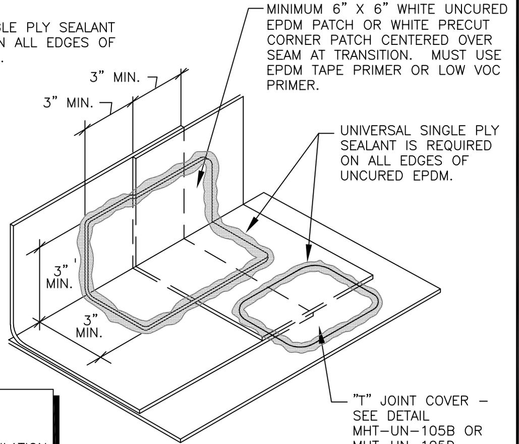
MINIMUM 6" X 6" WHITE UNCURED EPDM PATCH OR WHITE PRECUT CORNER PATCH CENTERED OVER SEAM AT TRANSITION. MUST USE EPDM TAPE PRIMER OR LOW VOC PRIMER.
