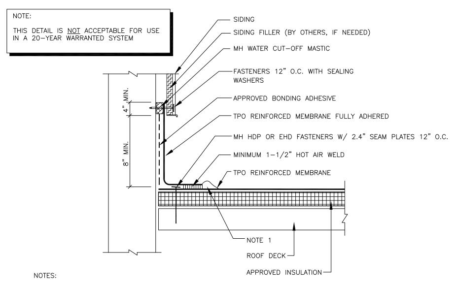
1. APPROXIMATELY 1 DIAMETER BEAD OF CUT-EDGE SEALANT IS REQUIRED ON CUT EDGES OF TPO REINFORCED MEMBRANE.
