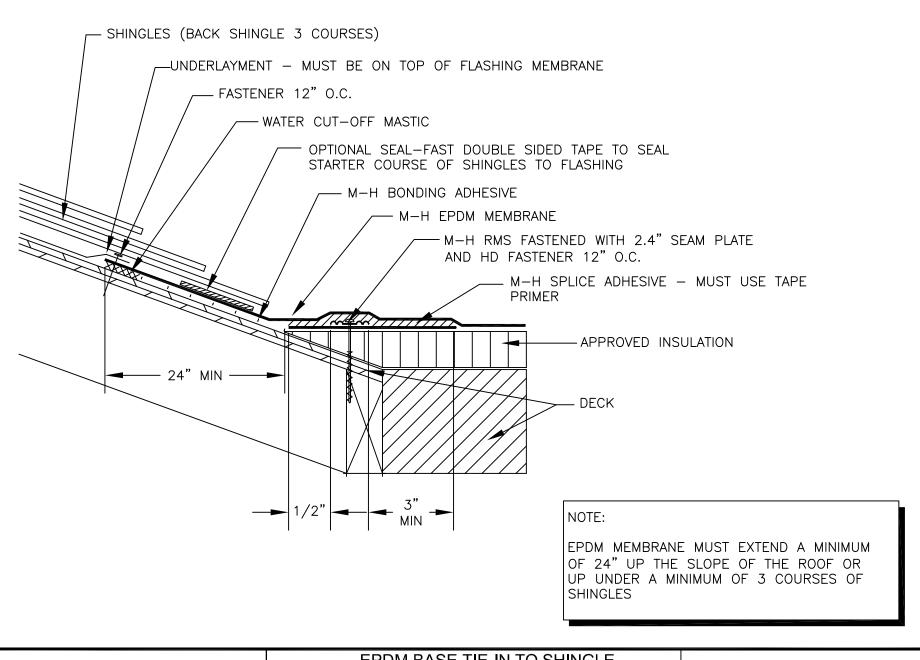
**MULE-HIDE** PRODUCTS CO., INC. **EPDM BASE TIE-IN TO SHINGLE ROOF WITH RMS** SYSTEMS:
