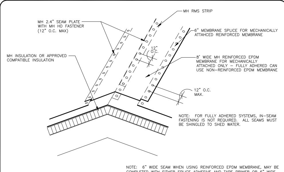
COMPLETED WITH EITHER SPLICE ADHESIVE AND TAPE PRIMER OR 6" WIDE IN-SEAM TAPE AND TAPE PRIMER.
